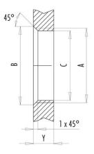
Installation direction: o-ring sits on chamfer.
